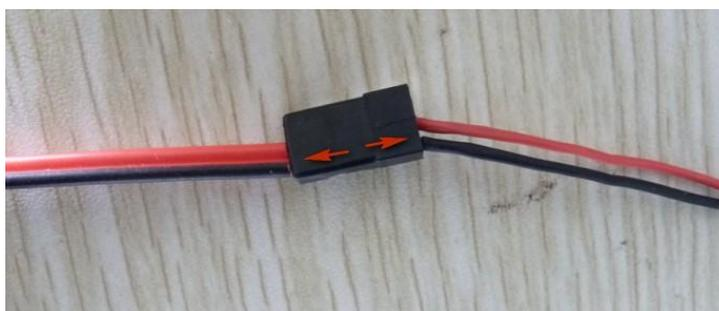
When you connect the Data radio to USB-TTL data cable, you need a 4P connecting wire like the picture below shows:
