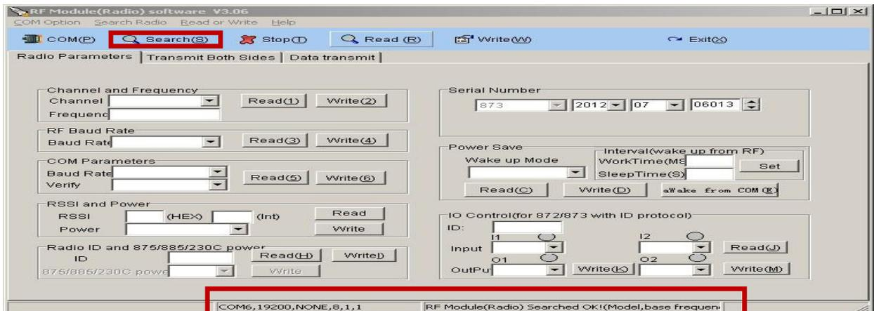
After detected the Data Radio, read the current various parameter values, you can choose "Read(R)" read all parameters, also you can click each item of the "read" readout parameters of this item:
