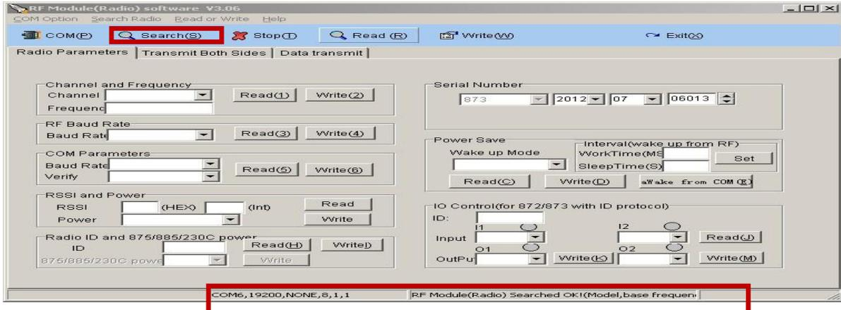
After detected the Data Radio, read the current various parameter values, you can choose "Read(R)" read all parameters, also you can click each item of the "read" readout parameters of this item:
