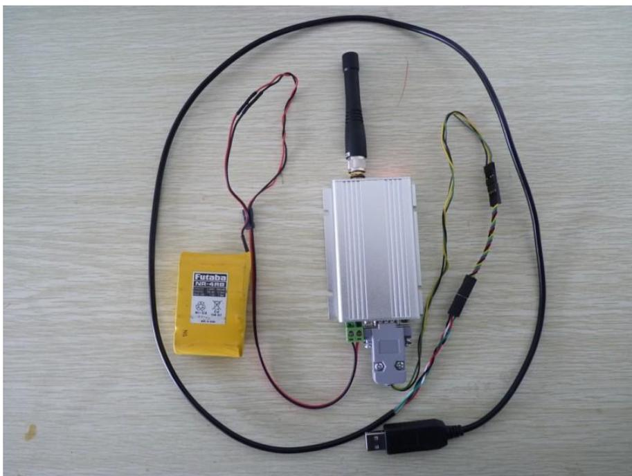
When you power on the Data Radio, the data radio data state LED will flash one time, and power state LED will stay on solid, like the picture below, the LED which is near the antenna is data state LED, and the one that stays on solid is power state LED:
