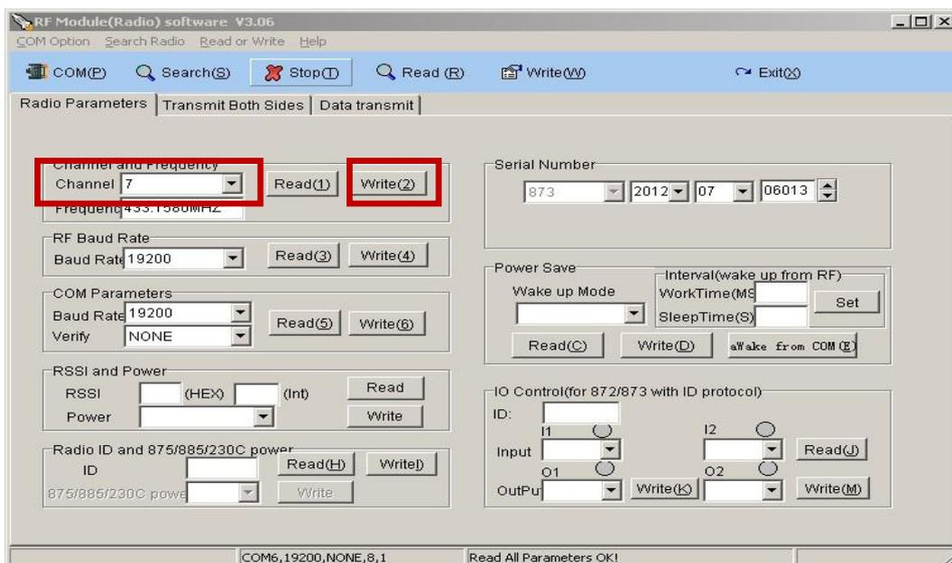
After configuration is "OK" ,please save the parameters to the Data Radio, otherwise the parameters will back to before after power off. Click on the "Write(W)", the software will save the parameters to the Data Radio, please re-detected again and read the current parameters, if the parameters
