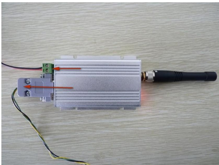
Like FY-602, the Data Radio will immediately into work state when it power on, so the antenna should be installed before power on, in order to avoid Data Radio frequency power amplifier circuit part overheat and burn out.
