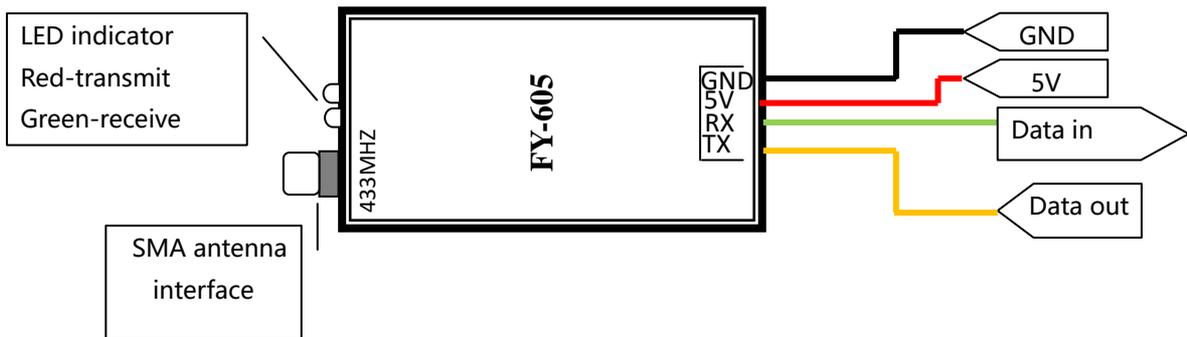
FY-605 is TTL level, interface default baud rate:19200bps .
