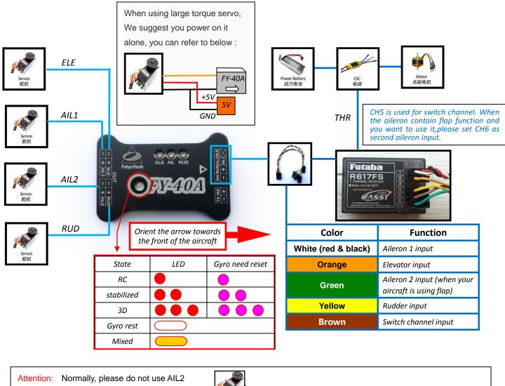
Attention: Normally, please do not use AIL2 port, just use a **Y cable** to connect two aileron servos to AIL1 port.
